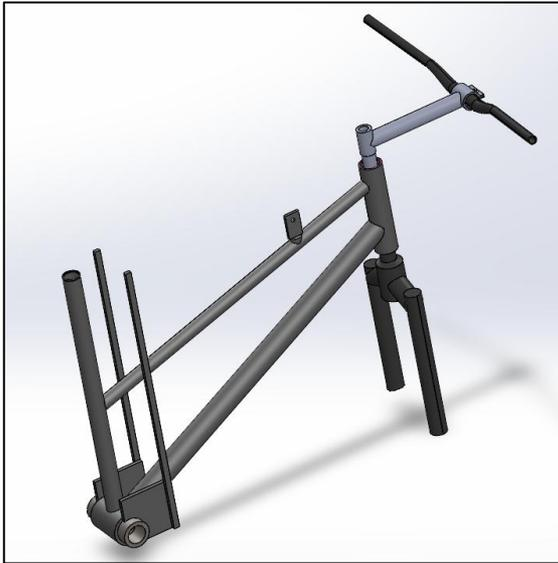
Figure 10: SolidWorks of Reused Parts (post modification)
