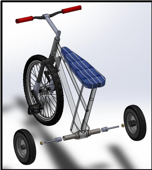
Figure 13: Final Design Exploded View
