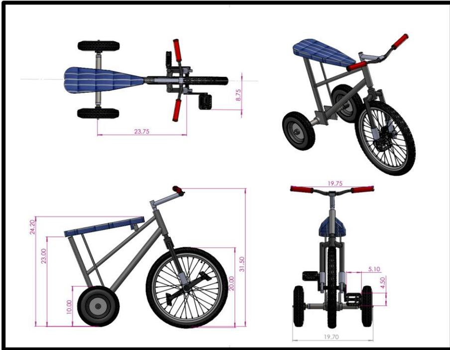
Figure 9: Final Tricycle Design Drawing
